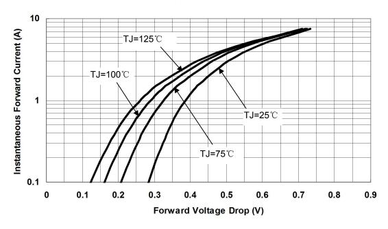
Fig.3-Typical Forward Voltage Drop Characteristics
