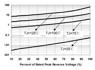
Fig.1-Typical Junction Capacitance
